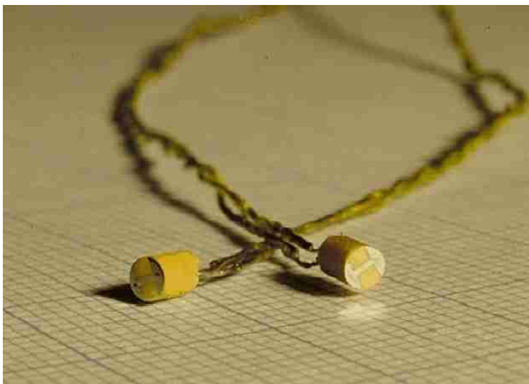
Thin Film Thermometer with connecting wires and cables
